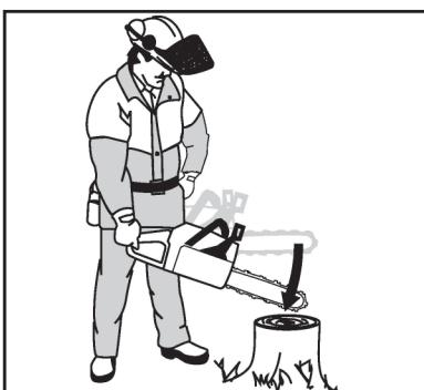
When the bar hits the stump the brake should be applied.
