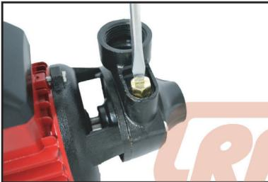
3. The water should be poured in through the priming plug.
