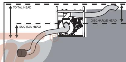
Pump output will be affected by the type, length, and size of the suction and discharge hoses.
