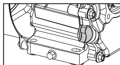
3. Turn the oil gauge dipstick/cap counterclockwise, remove it and clean it with a clean cloth.
